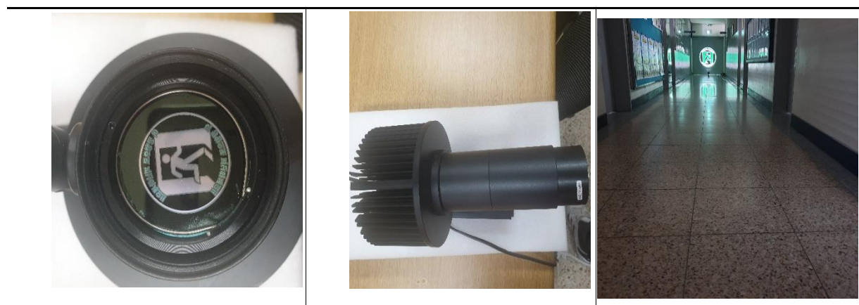
(a) Display surface of image output emergency lighting
