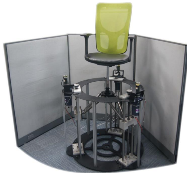
Figure.6. showing the outlook of the developed motion simulator
