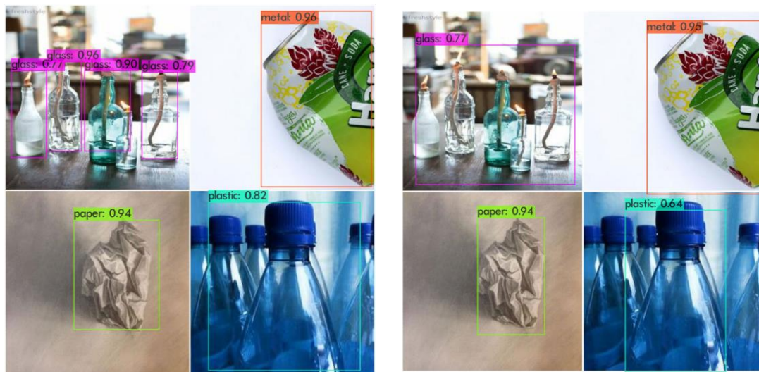
Figure 8. Testing Input Images Using Google Colab (a) YOLOv4 dan (b) YOLOv4-tiny
