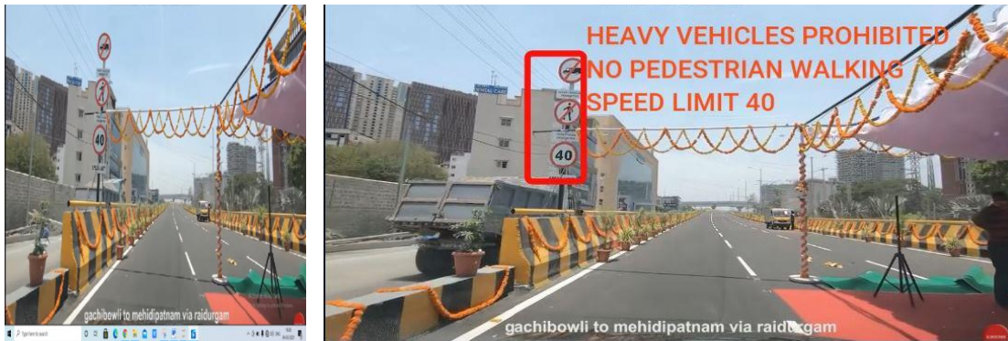
Figure. 5: Result of Traffic Sign Detection (on left) Input video (on right) Traffic Sign detection
