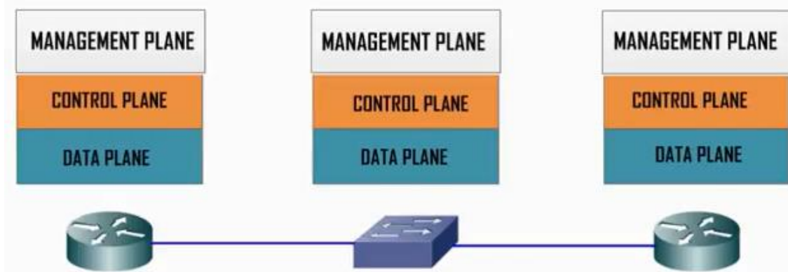
Figure 2. Every networking device has its management plane, control plane, and data plane.
