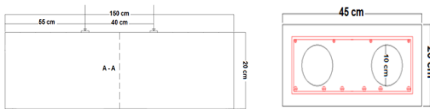
Figure 2. Hollow-core slabs specifications
