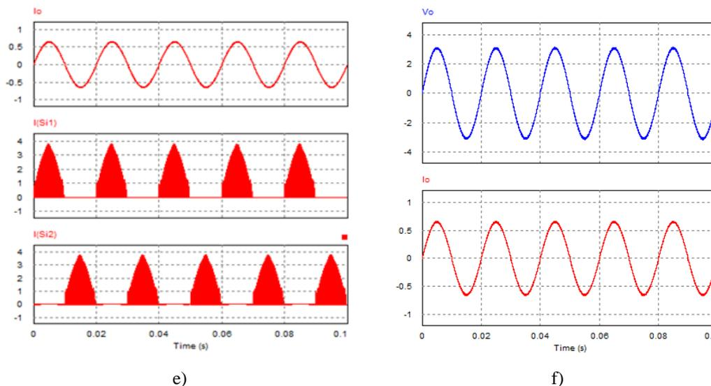
**Fig. 4.** a) Waveform pulses of switch gates, b) Voltage and current waveform of main diode Di1, c) Current waveform Lr1 and voltage Cr, d) Current waveform of switch Si1 above and its zoomed state at the bottom, e) Output current waveform at the top, Si1 current in the middle and Si2 current at the bottom, f) Output voltage waveform at the top and output current at the bottom.
