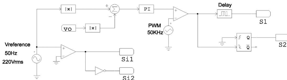
Fig. 2. Converter switch control circuit.
