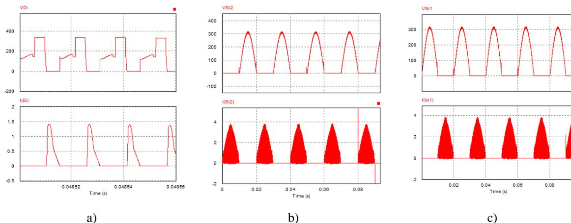
**Fig. 6.** a) Diode voltage and current waveform Di, b) Si1 switch voltage and current waveform, c) Si2 switch voltage and current waveform.
