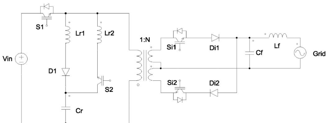
**Fig. 1.** The proposed ZCT flyback microinverter.
