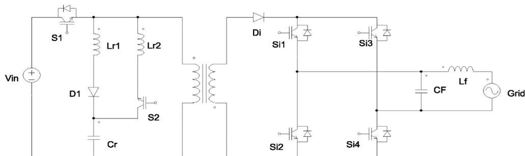
Fig. 5. Flyback microinverter using a four-switch inverter.
