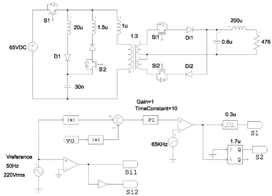
Fig. 3. General schematic of converter simulation in PSIM software.
