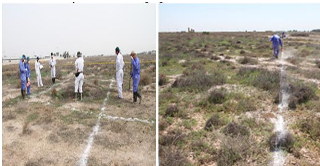
Figure.6.A grid system for survey of site grounds
