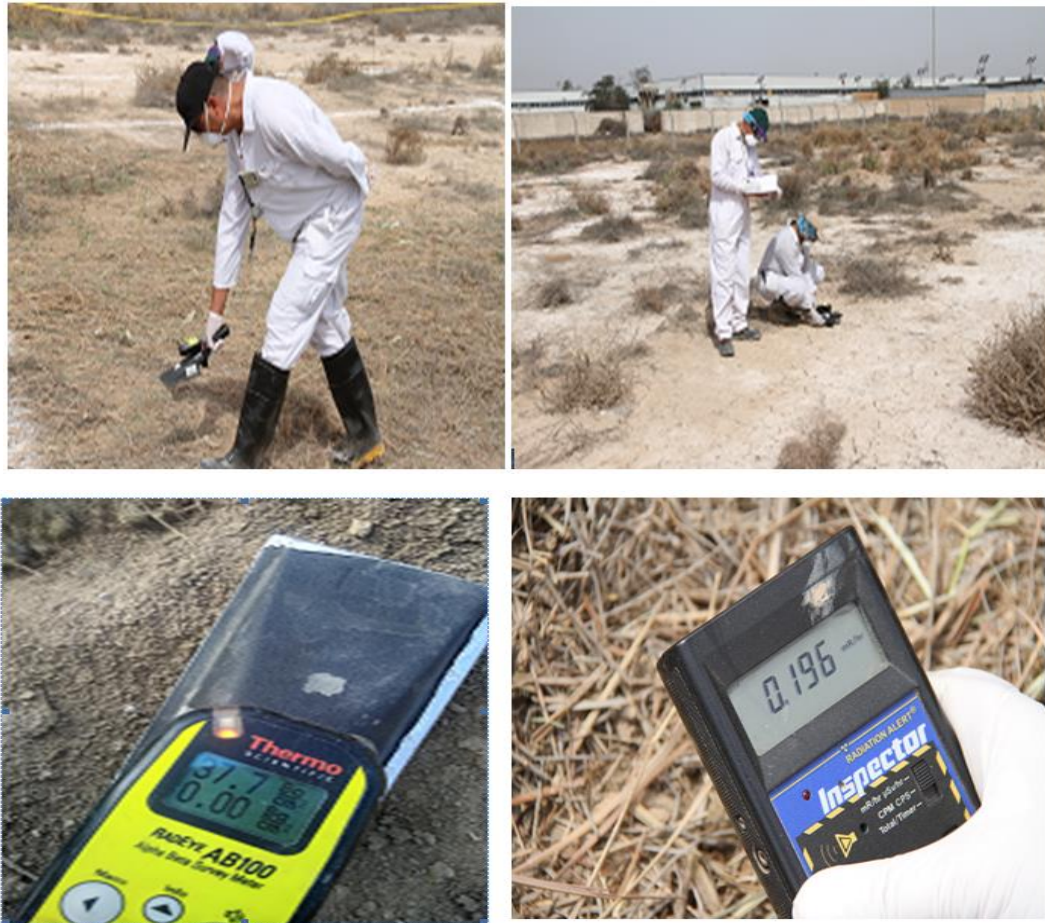
Figure.7. Radiological survey the contaminated site with documentation with radiation measurements
