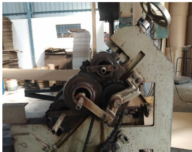
Fig.10. Corrugator machine flutes (side view)
