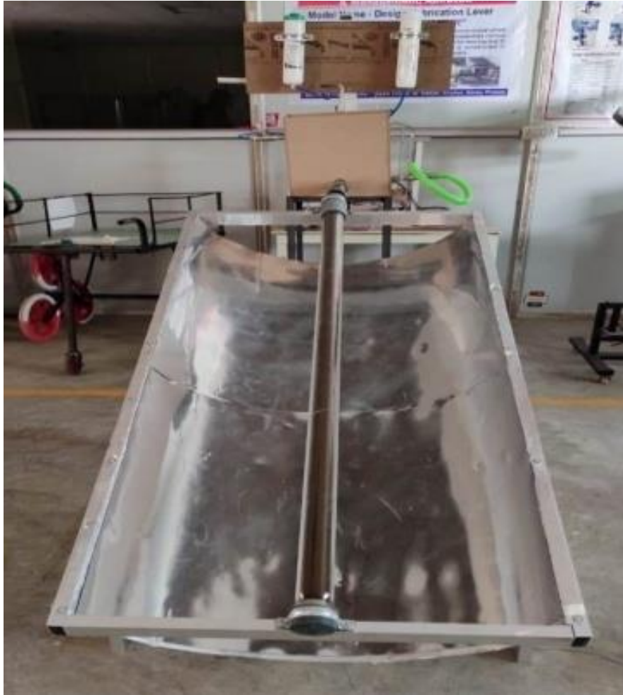
Fig 2: solar water purifier with evacuated tube and carbon filter
