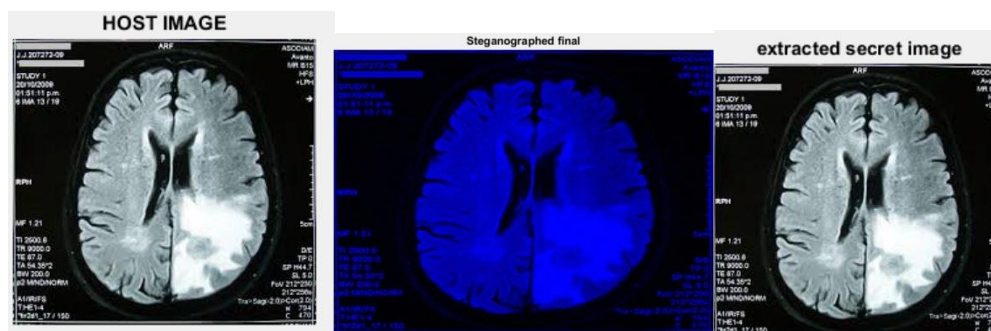
Fig7(a): Host Image Fig7(b): Watermarked Image Fig7(c): Recovered Image Fig7: Experimental results of watermarking on brain tumor diagnostic image
