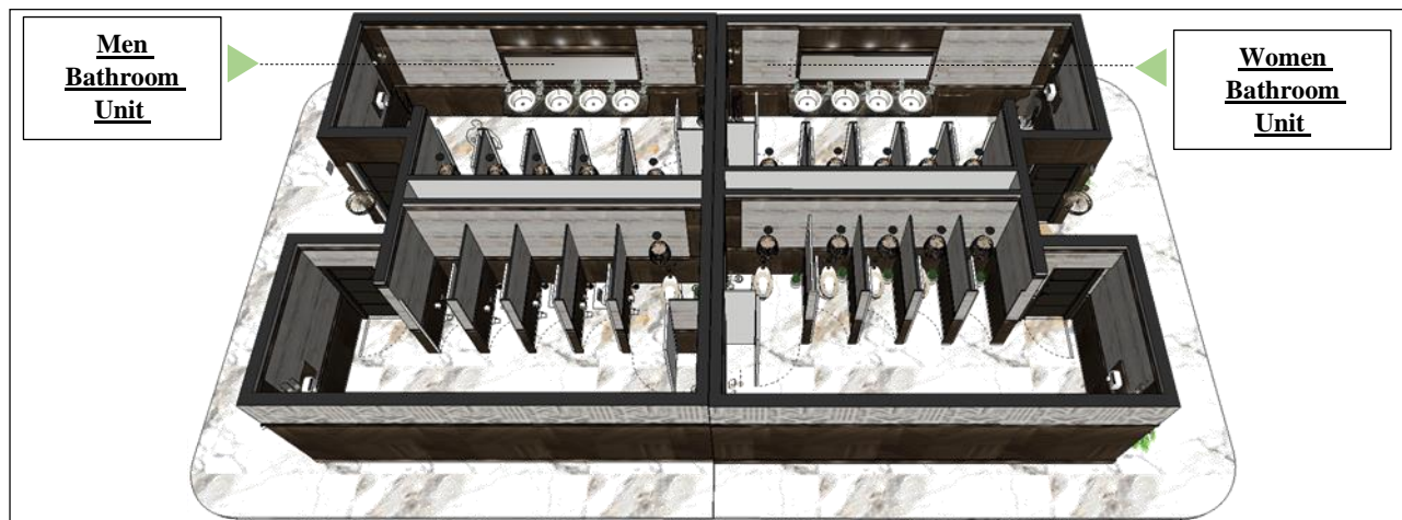
Figure 32. Top Perspective of Bathroom Unit.
