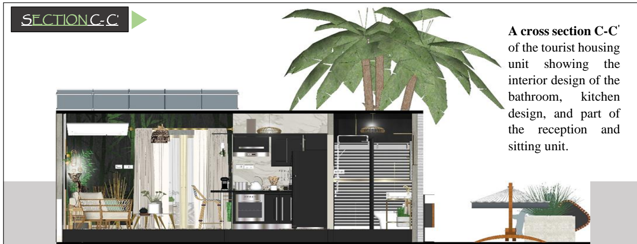
Figure 11. Section C-C' for Tourism Housing Unit.
