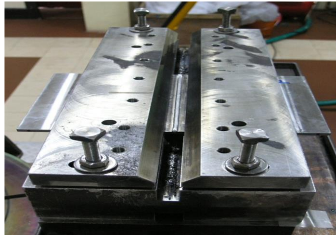
Figure 1. Machine of Inconel 718 Alloy plates used for Electron beam welding
