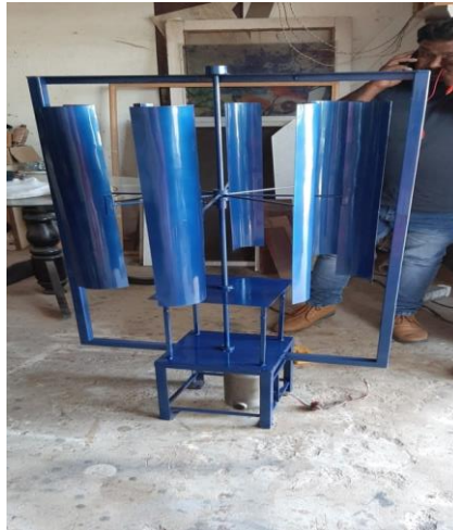
Figure 1 Vertical Axis wind Turbine with color coating
