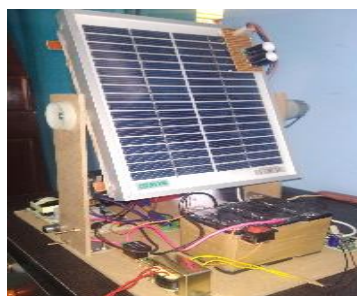
Fig 2: Automatic Solar tracker induction motor drive
