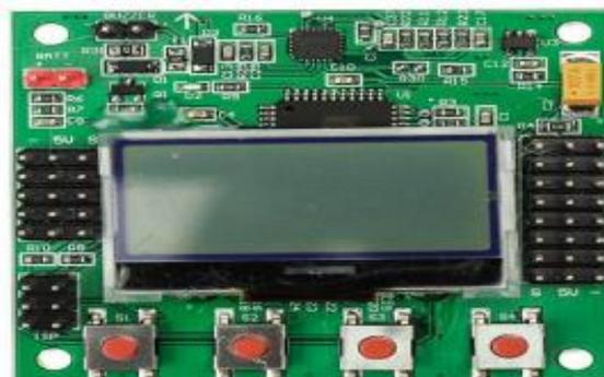
Fig 2: Flight Controller Board
