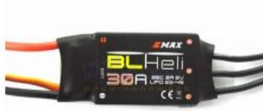
**Fig 3:** Electronic Speed Controller
