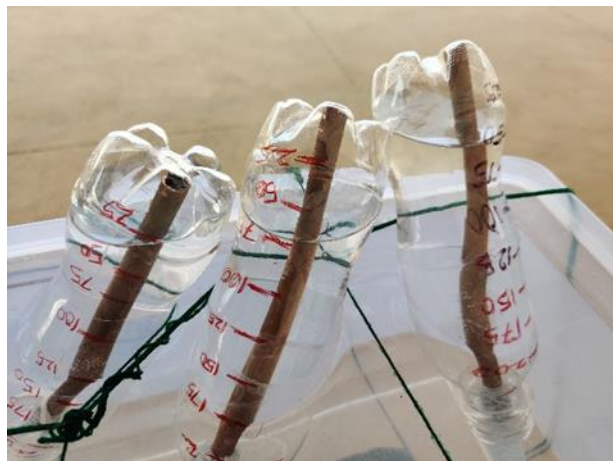
Fig J – The collection vessel shows the gas collected with their quantities.
