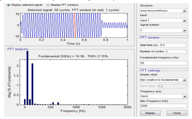
Fig.12 Source current THD with proposed controller is 2.15%
