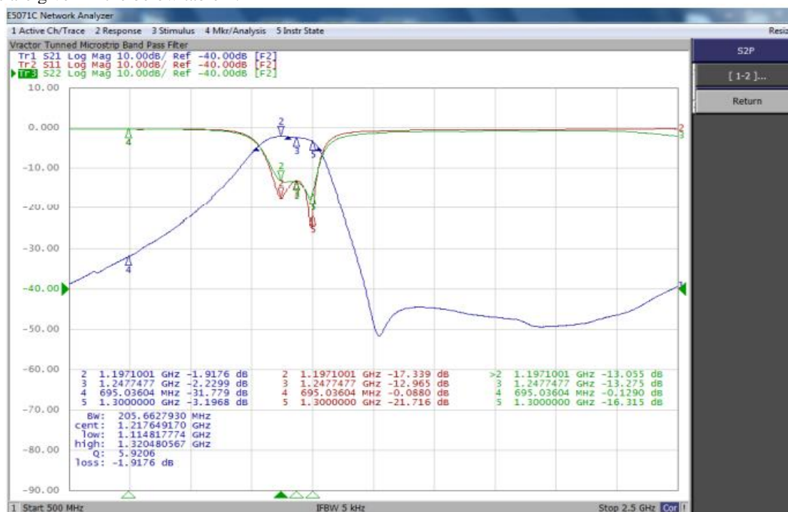
Fig.6: Frequency response of Bandpass Filter at 1.21GHz in Network Analyzer.
