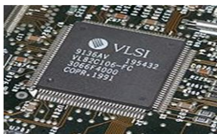
Figure: 1 A VLSI VL82C106 Super I/Ochip
