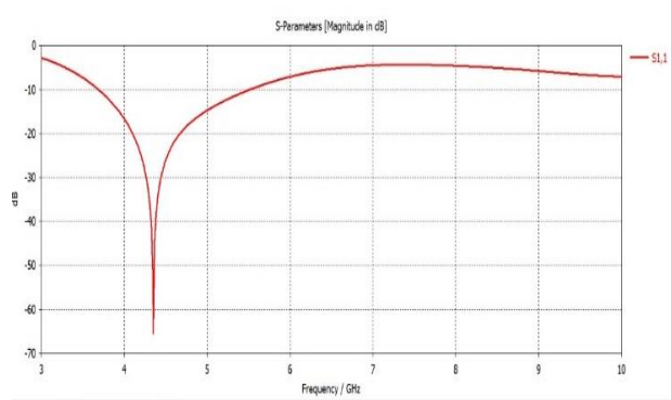
Fig.2. The Return loss of the individual patch antenna
