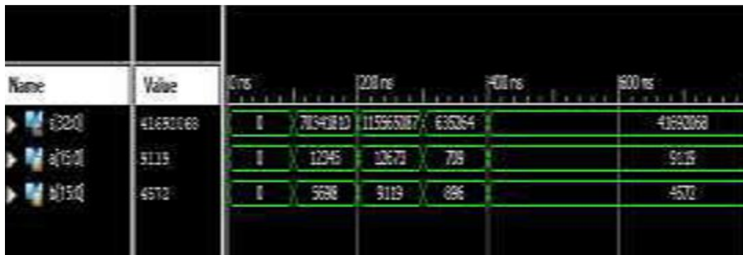
Fig-6: Exact simulation result for 16x16 multiplier
