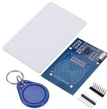
Figure 5: RFID Reader & Tag
