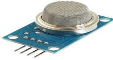
Figure 6 Gas Sensors for Air Quality
