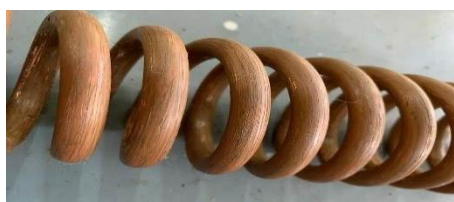
Fig. 2. Surface Modified coil
