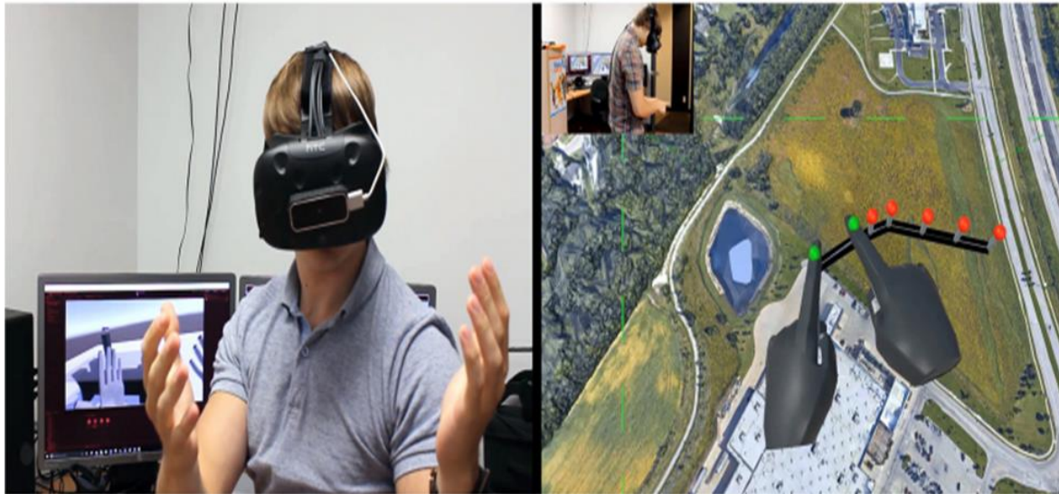
Figure 3. Set-up showing the Leap Motion device affixed onto an HTC Vive VR headset (Left). Virtual hands (on-screen) positioned in VR in place of the real user's hands (Right) [54]
