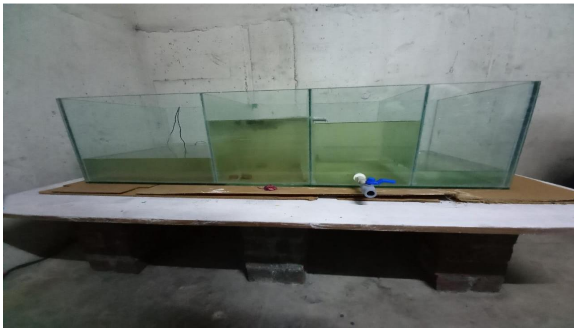
Fig. 2 Fluidized Bed Reactor in Sewage Treatment Plant
