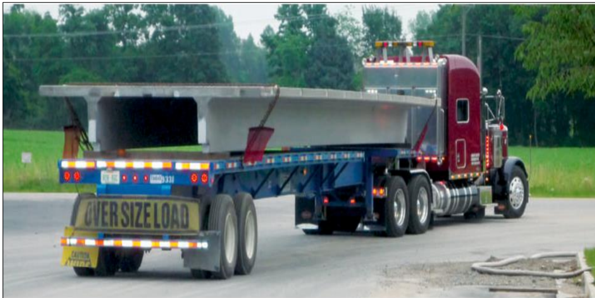
Figure 6: Shipping DT to project site (PCI Design Handbook, 2017)
