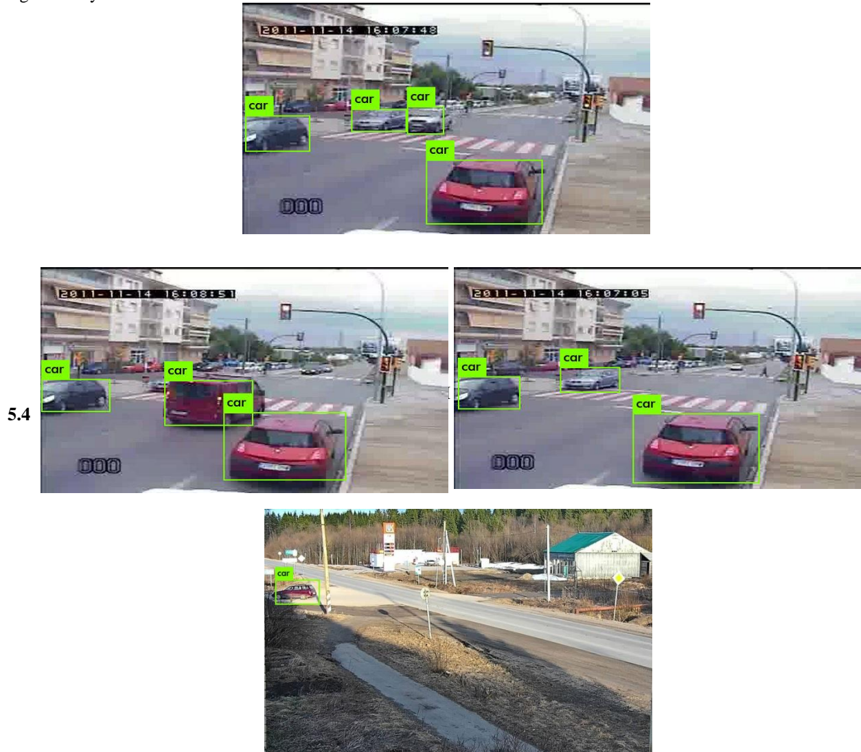
Fig 10 Detection of vehicles in a CCTV video. Right – A small car is undetectable by the detector
