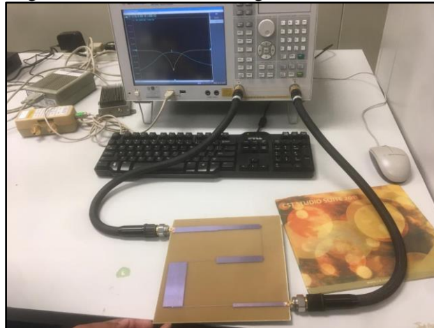
Figure 7: The laboratory experimental for the fabricated Band Pass Filter
