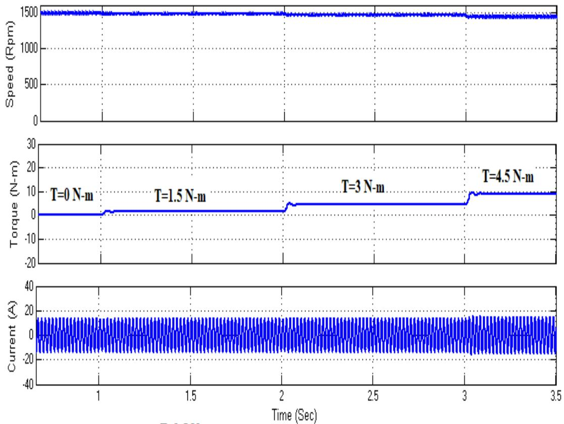
Figure 8. Output waveforms of speed, torque, and current.
