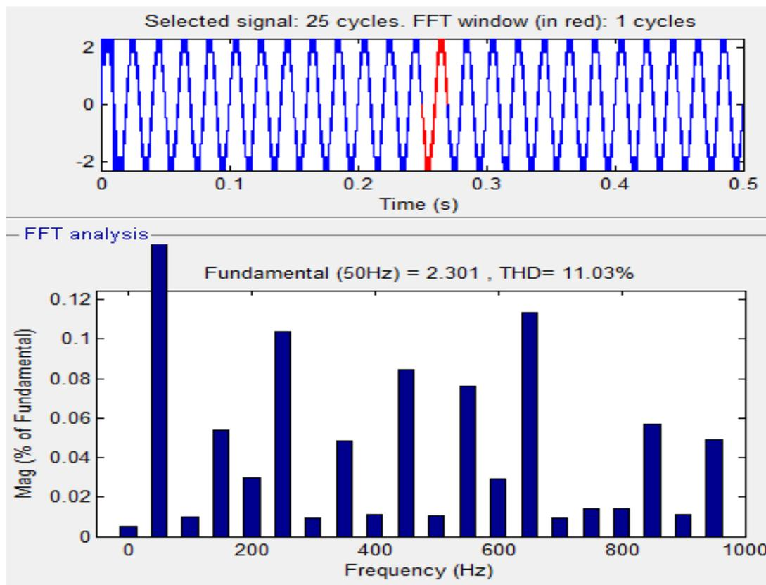
Figure 17. Eleven-level inverter source current THD plot
