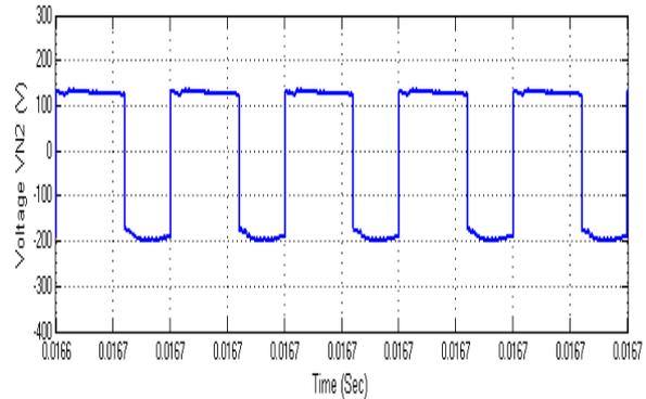
Figure 3(b). Secondary voltage  $V_{N2}$ (V)
