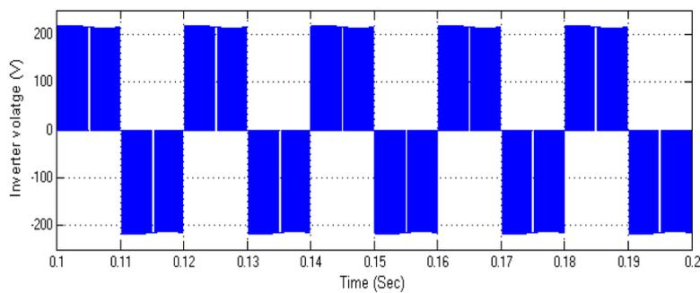
Figure 4(a). Output voltage
