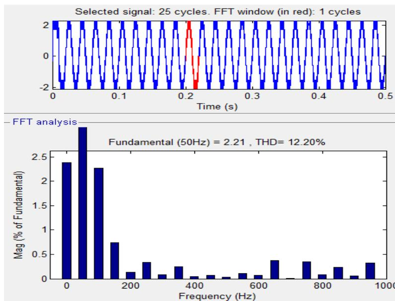
Figure 15. Source current THD plot for 9-level inverter
