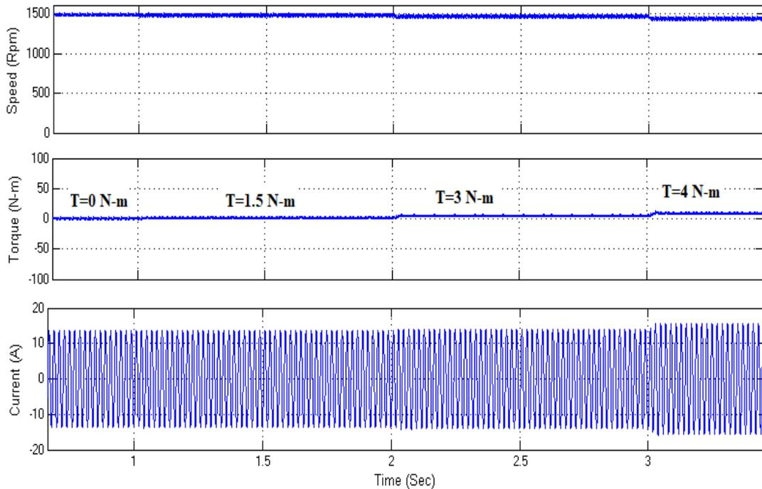
Figure 14. Output waveforms of speed, torque, and current at different loading conditions of 9-level inverter
