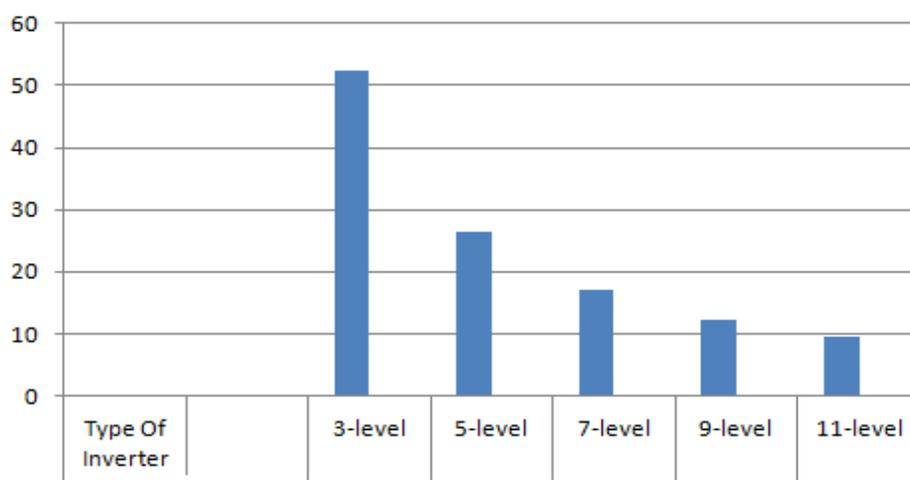
Figure 18. Graphical representation of source current THD at different levels
