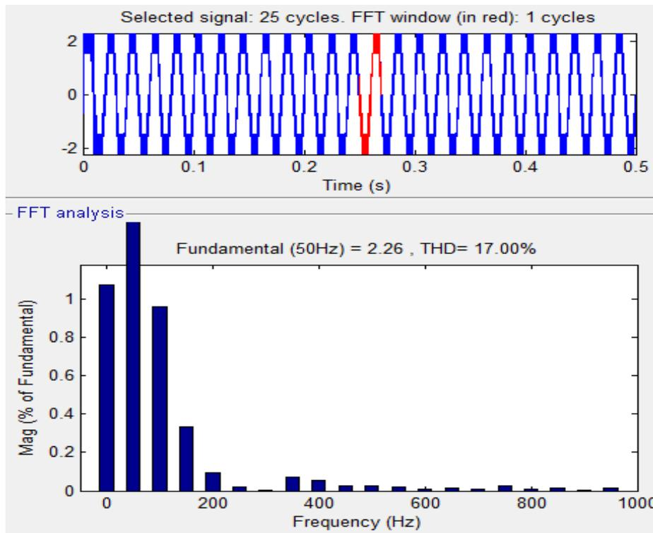
Figure 12. THD plot of 7-level H-bridge multilevel inverter
