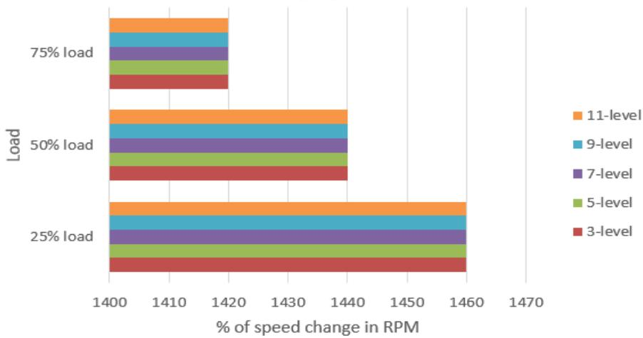
Figure 20. Representation of speed at different loading conditions with different multilevel inverters
