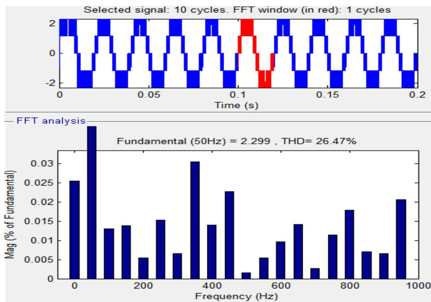
Figure 9. THD plot 5-level H inverter source current
