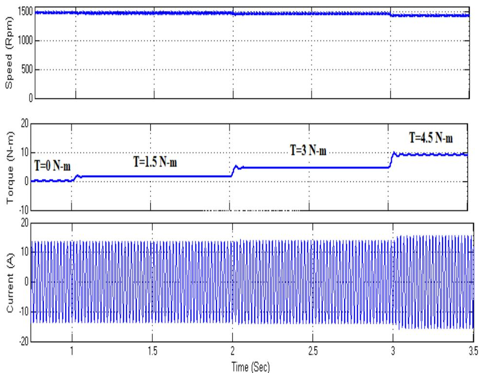
Figure 16. Output waveform for Speed, Torque and Current at different loading conditions 11-level inverter
