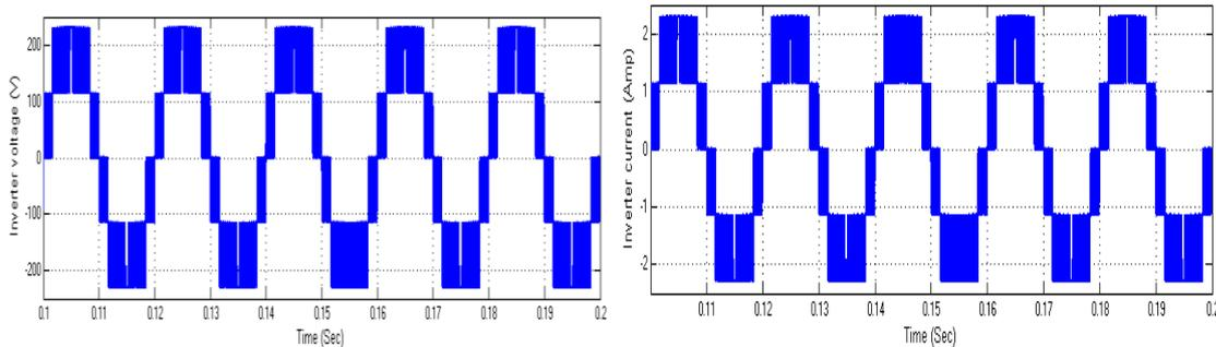
Figure 7(a). Output voltage.
