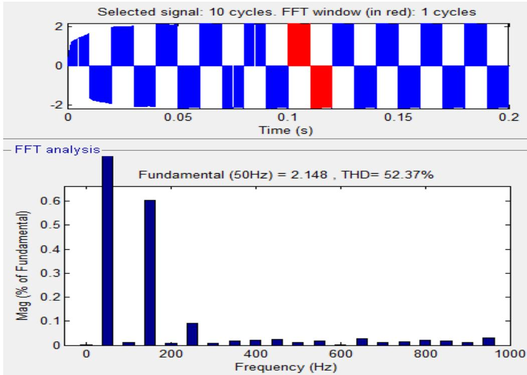
Figure 6. Three-level inverter THD
