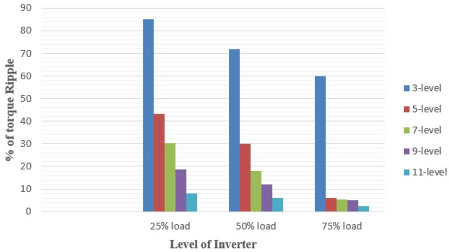
Figure 19. Graphical representation of %torque ripple at different loading condition with different levels
