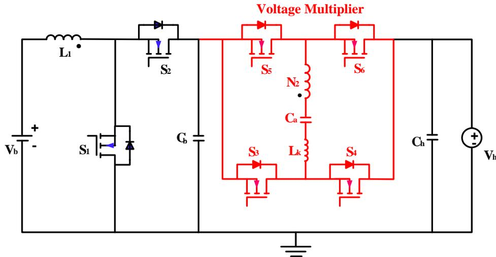
Figure 1. Step-up converter integrated with voltage multiplier
