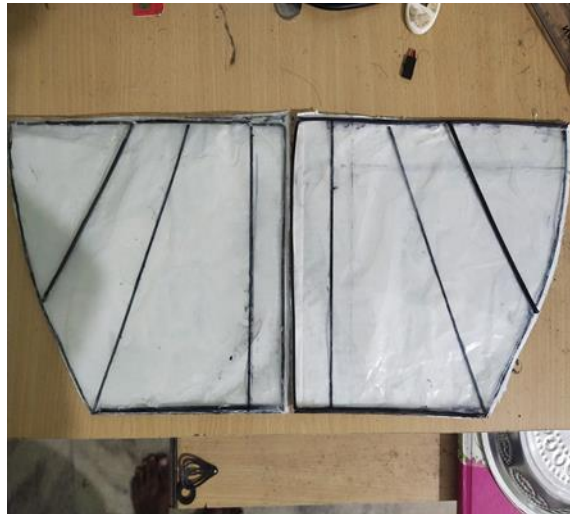
Figure 2.7 Fabricated Orcon Flat Wing
