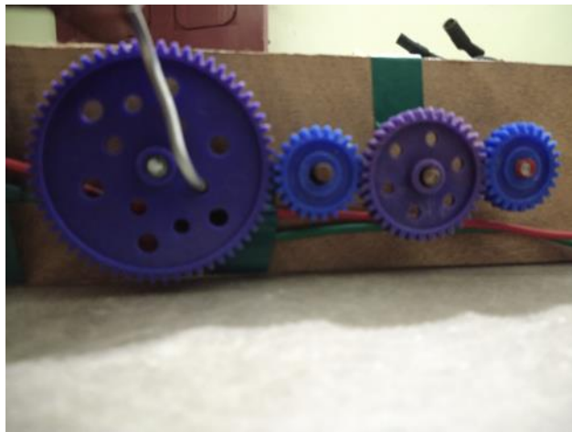
Figure 2.8 Gear Setup For Ornithopter
