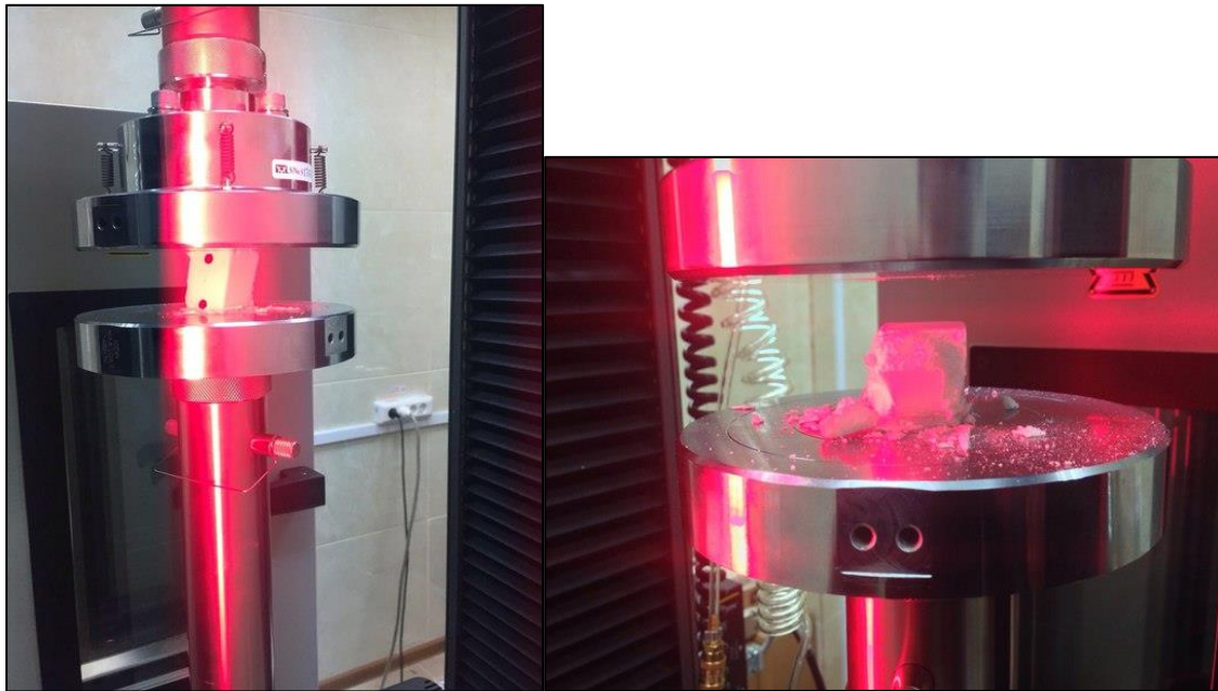
Fig. 5. Loss of stability of the sample. Sample destruction.
