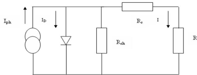
Figure 2. PV cell Configuration
