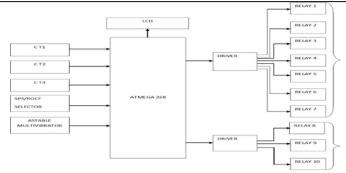
Figure 1. Block Diagram
