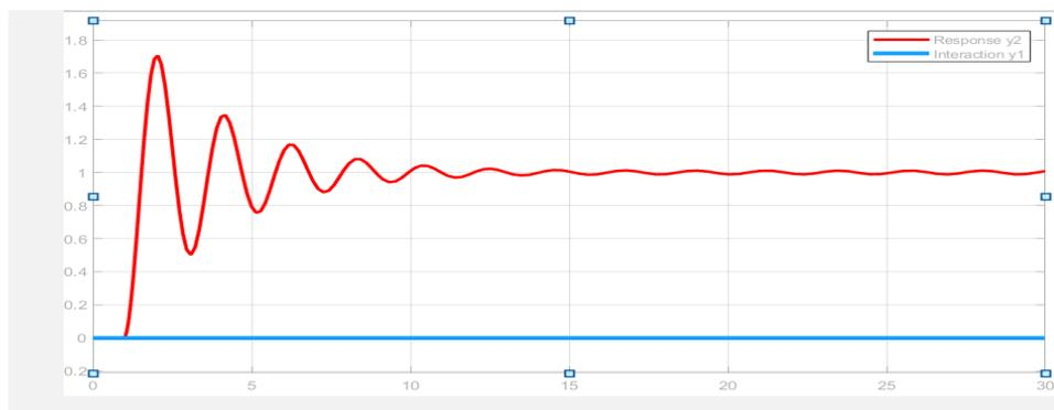
**Figure 2:** PI Controller output with different decouplers for a phase input in  $y_1$  and  $y_2$ .
