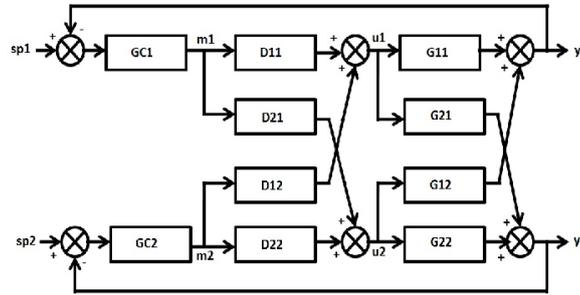
Figure 1: Decoupled TITO Process
