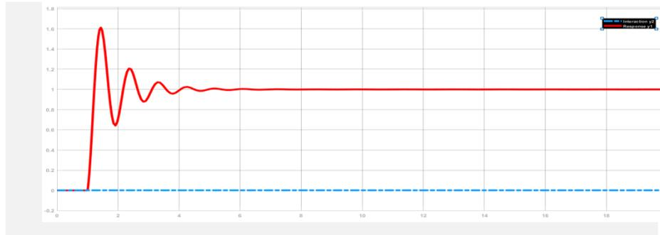
**Figure 3:** The dual-loop controller's responses for a phase input in  $y_1$  and  $y_2$ .
