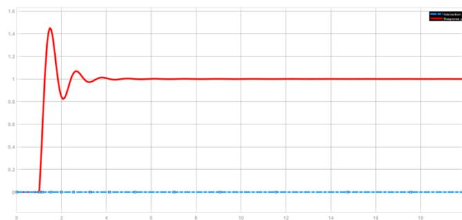
**Figure 3** shows the dual-loop controller's responses are far superior to a one-loop PI control system. Here the loop-interactions are considered to be marginal and the second control is tuned for setpoint-tracking.
