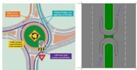
Fig 3. Showing the U-turn and Rotary junction
