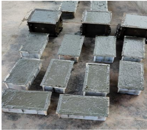
Fig.4 Casted Rectangular paver blocks and cubes
