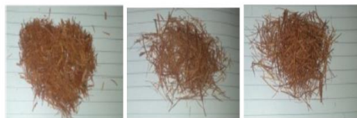
Fig. 1 Coconut fibre of 10mm, 15mm & 20mm Length.
