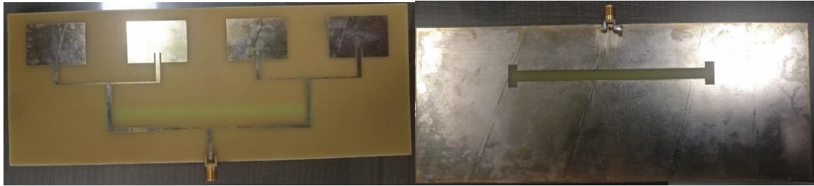
Fig 1.24- 1 x 4 Element MSPA Array Patch with DGS Fig 1.25- 1 x 4 Element MSPA Array with DGS Ground
