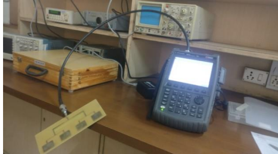
Fig 1.27 – Testing of 1 x 4 Array MSPA with DGS
