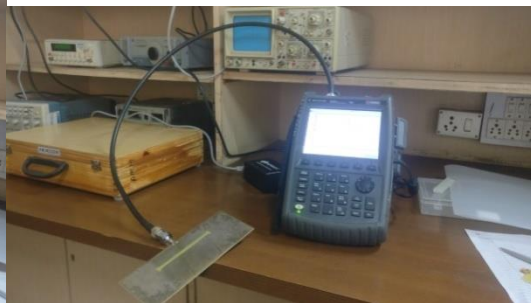
Fig 1.28 – Testing of 1 x 4 Array MSPA with DGS
