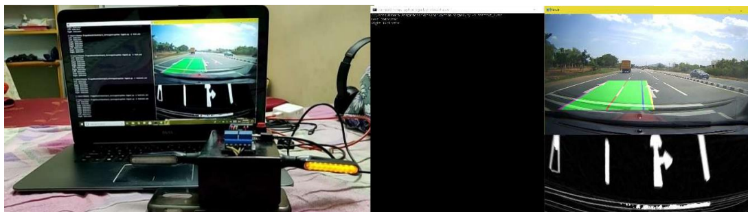
Figure 20. Wrong lane line detection
