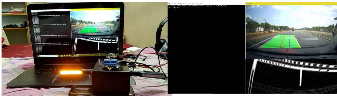
Figure 19. Misalignment of lane line
