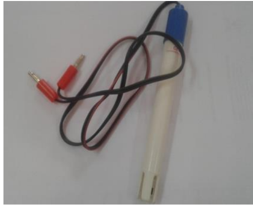
Figure 6. Probe to Sense Electrical Conductivity
