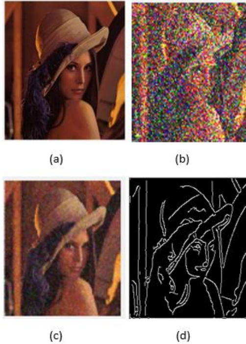
Fig.5. (a) Original lena image (b) Image with Gaussian noise (c) Denoised image by applying nonlinear prefiltering (d) Edge image obtained by applying distributed canny edge detector block by block on denoised image in (c)
