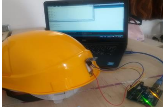
Angle variation is detected using Gyroscope
