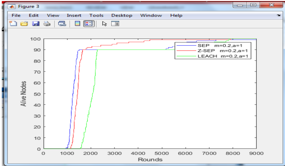
Figure 11. The number of alive nodes against rounds for LEACH, Z-SEP, and SEP.
