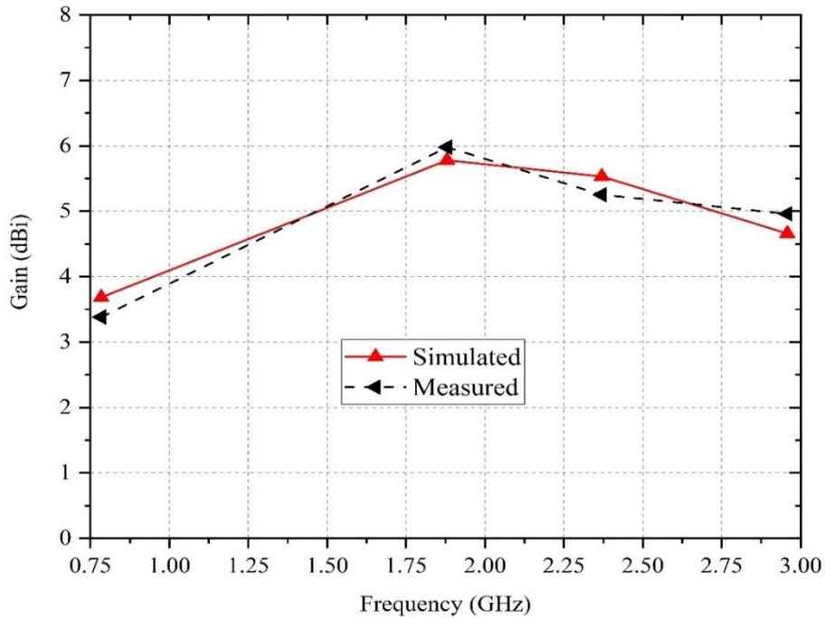
**Figure 4.** The comparison between simulated and measured peak realized gain of the antenna.
