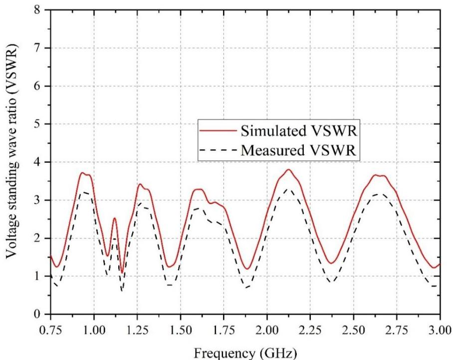
**Figure 5.** The comparison between simulated and measured VSWR of the antenna.
