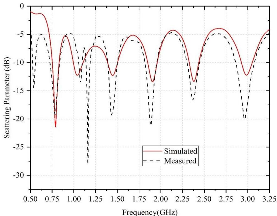
**Figure 3.** Comparison between simulated and measured scattering parameter (S11) of the proposed antenna.
