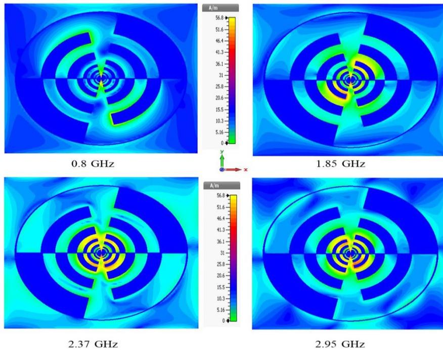
Figure 6. Current distribution at different frequency bands.
