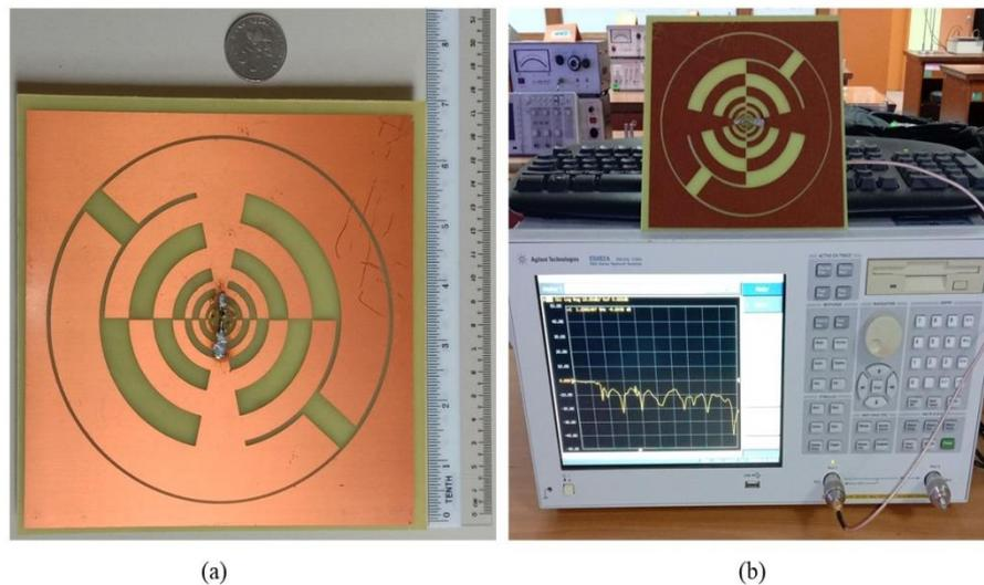
**Figure 8.** The measurement setup in the lab environment, (a) prototype image of the proposed antenna, (b) measured RL result.
