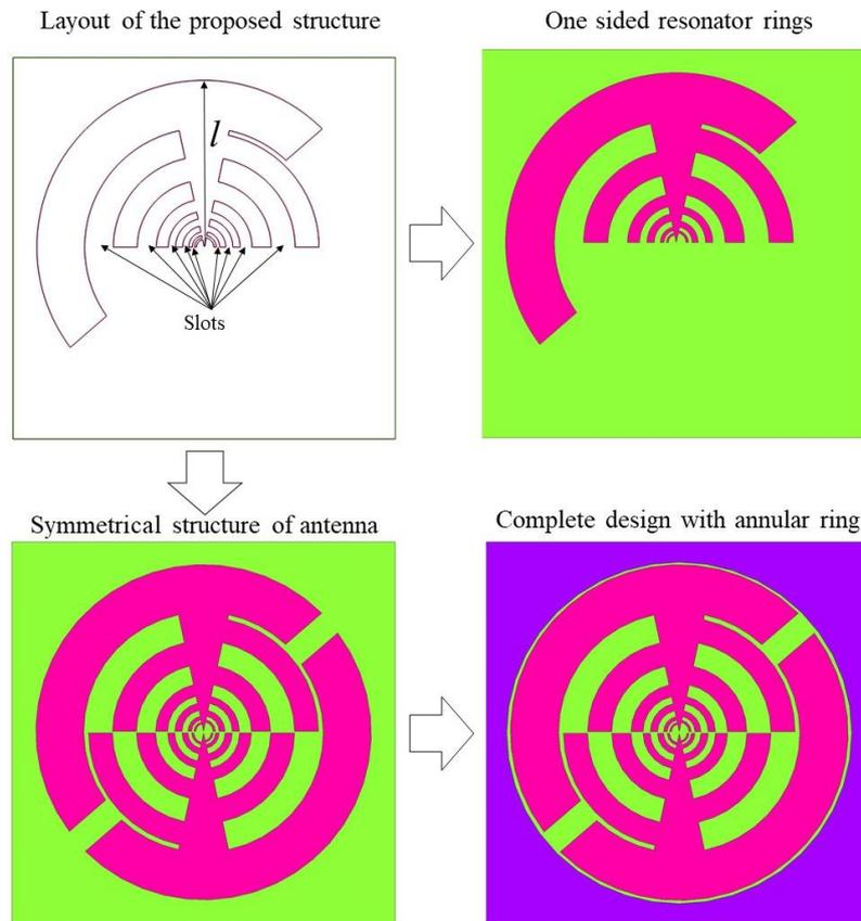
**Figure 1.** The sequential design process of the proposed antenna, a two-armed log-periodic self-complementary ring-turnstile shape with a discrete port and annular ring structure.
