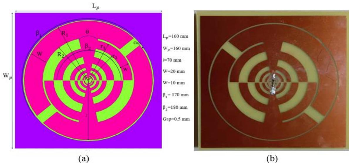
**Figure 2.** (a) The geometrical view with the optimized dimension of the proposed antenna, (b) prototype image of the proposed antenna.
