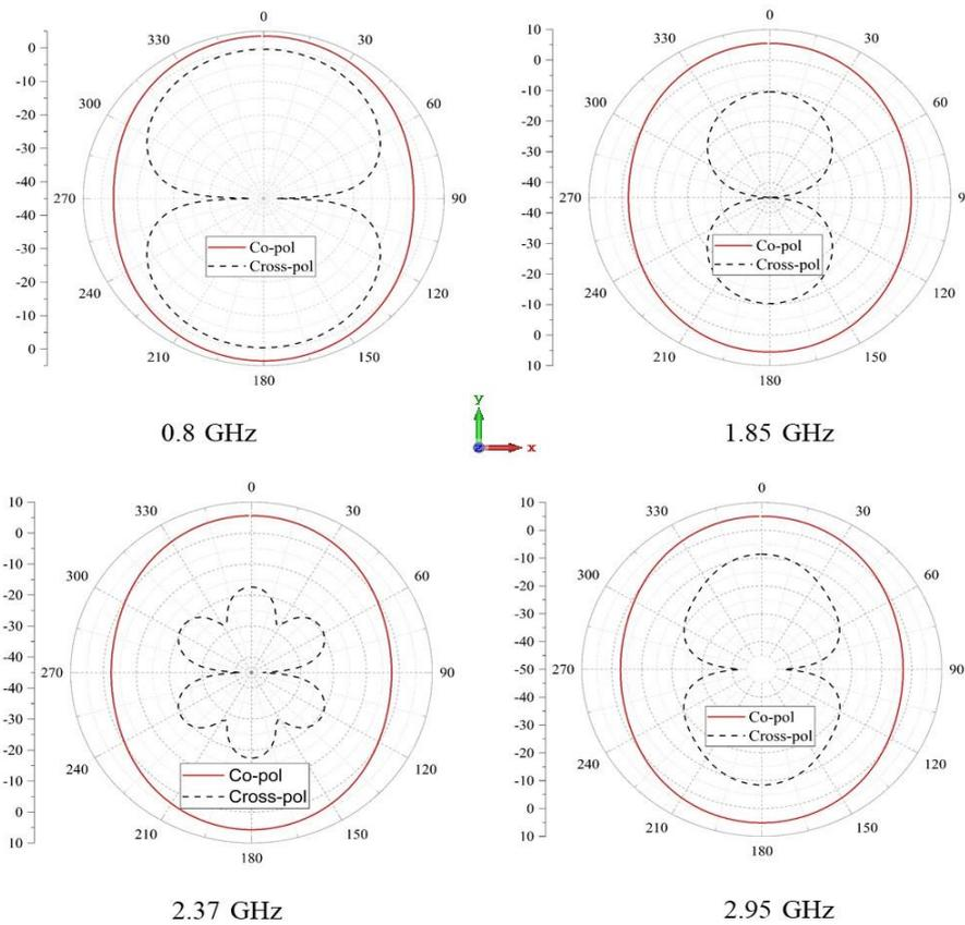
**Figure 7.** Directivity radiation pattern in polar form for different resonant frequencies.
