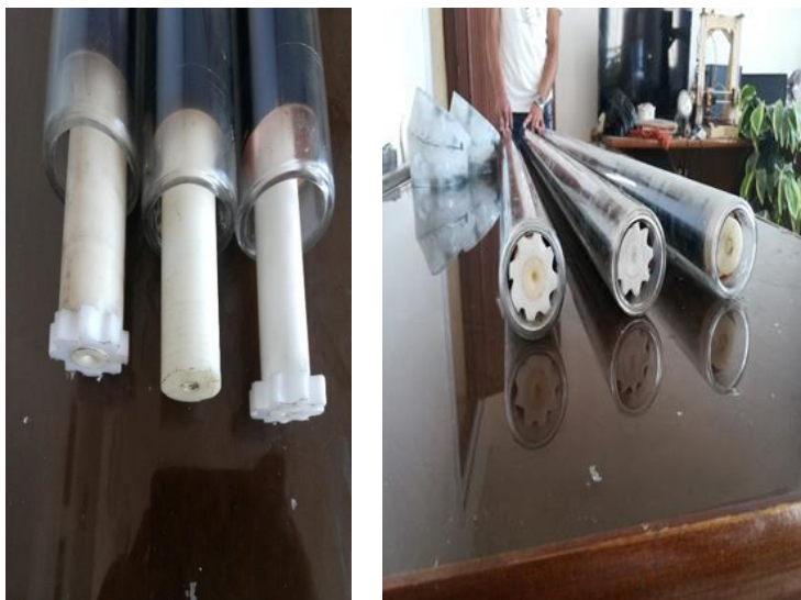
Fig. 4 Pictures of ERTALON columns inside the ETCs
