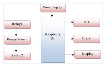
Figure.2.System Design Block Diagram
