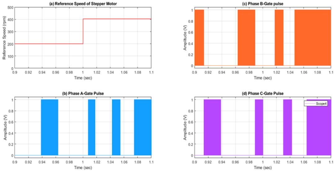
Fig. 8. Generated PWM signals for the Driver Circuit
