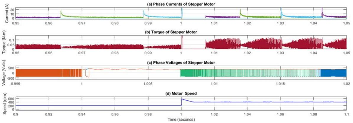
Fig. 9. Response of 3-phase stepper motor.
