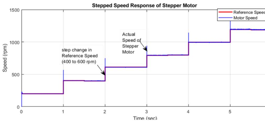
Fig. 7. Stepped speed response of stepper motor.
