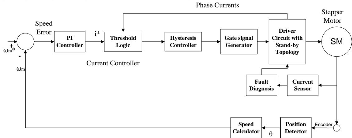
Fig. 2. Closed loop control system for stepper Motor drive.
