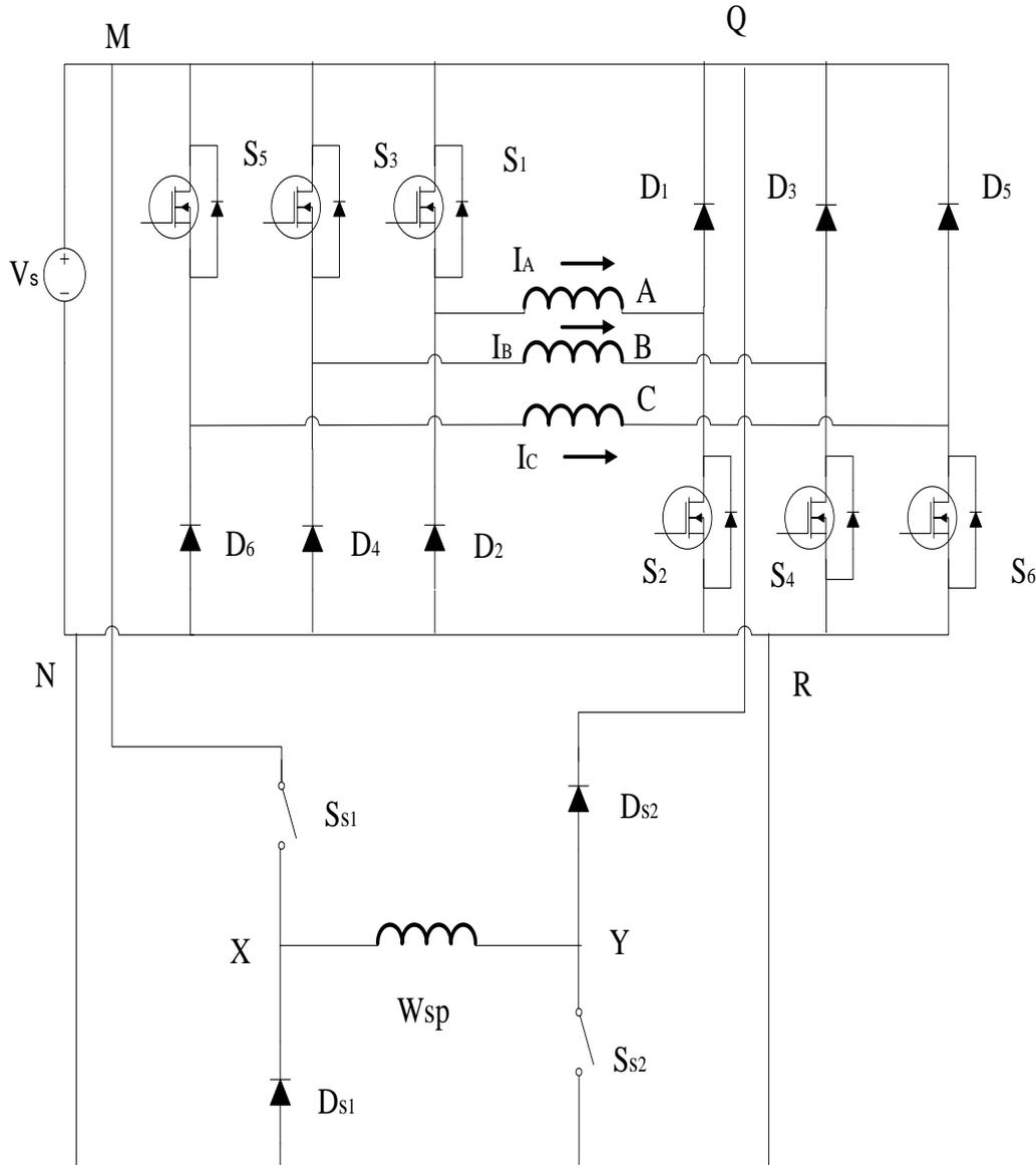
Fig. 3. Fault Tolerant topology for Stepper Motor Drive.
