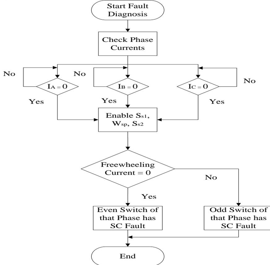
Fig. 5 Flowchart of the SC fault
