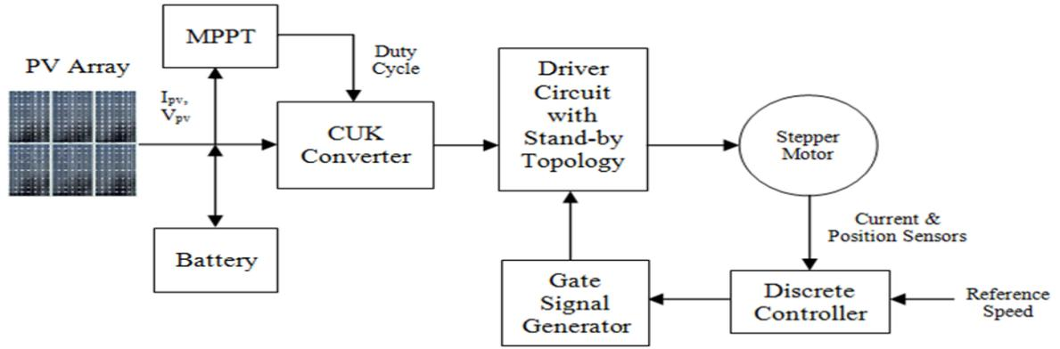
Fig. 1. Block diagram of PV fed stepper motor drive.
