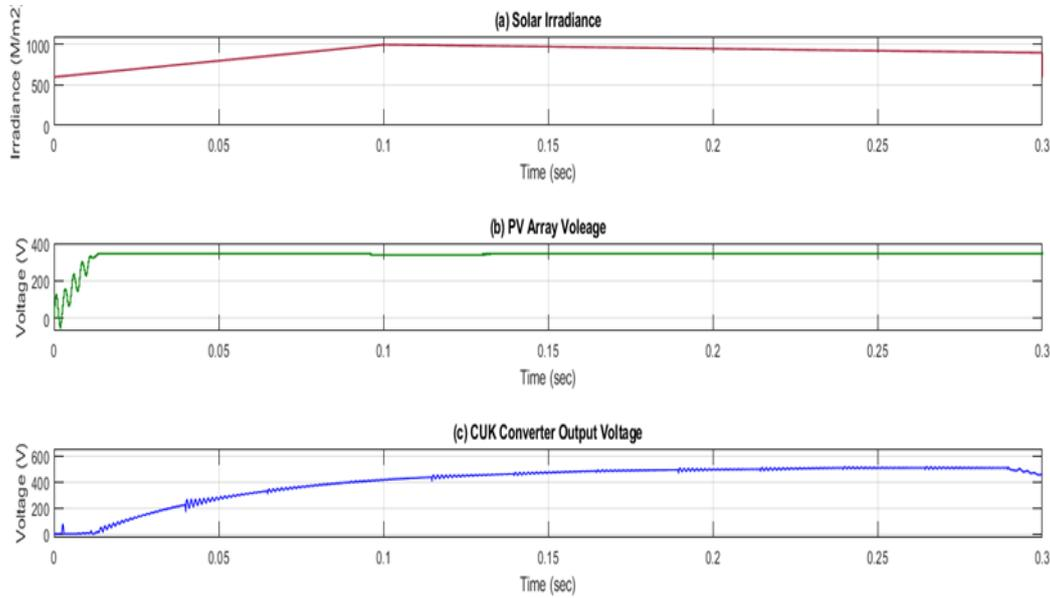
Fig. 6. PV Array Response and Converter Output Voltage
