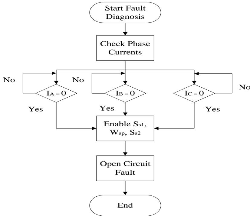
Fig. 4 Flowchart of the OC fault detection topology
