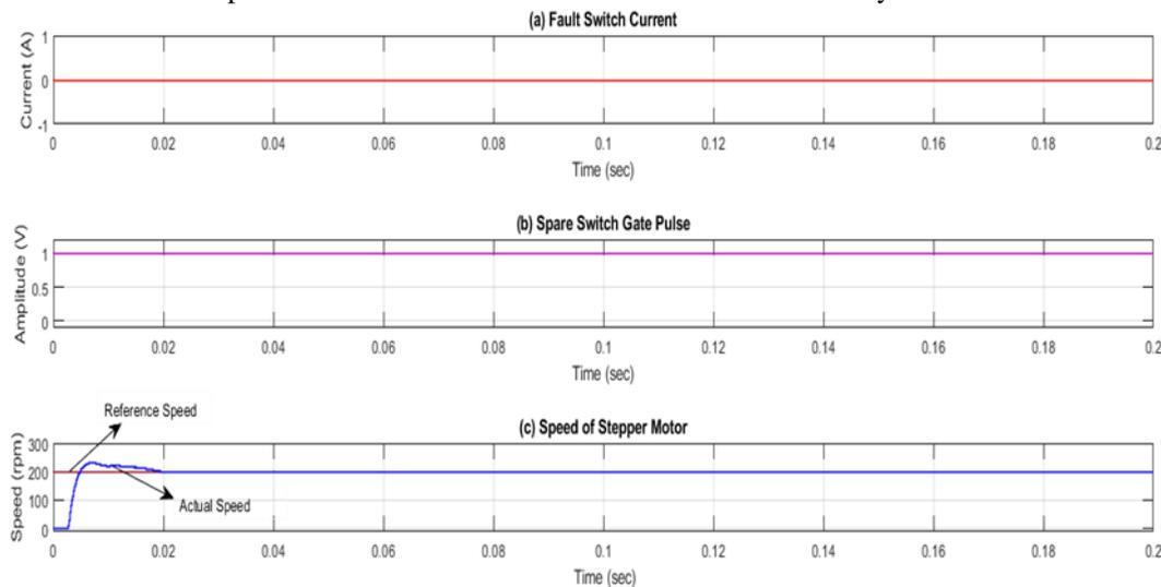
Fig. 11. Response under Fault condition
