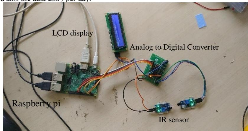
Figure 2. Hardware Setup of Proposed System
